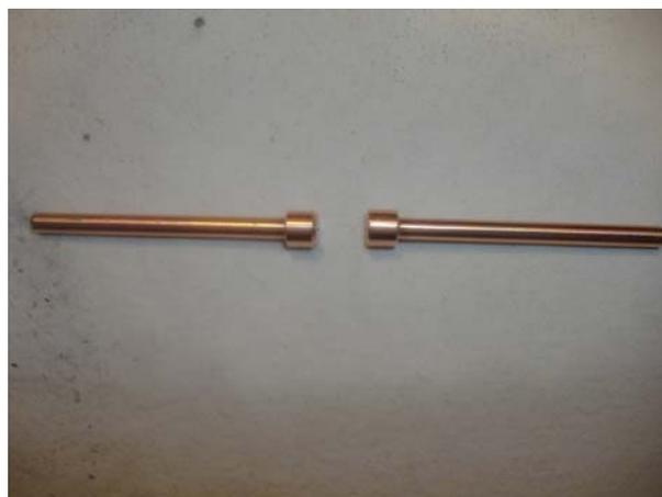
ELETTRODI DI RAME TORNITI
